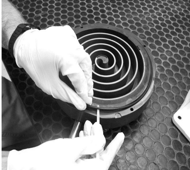
7. Remove the old tip seals from both the outboard housing and orbiting plate.
