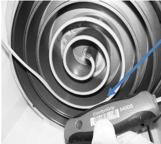
11. Finish installing the rest of the tip seal and using a set of cutting pliers, cut the tip seal leaving a 1/8<sup>th</sup>-inch or 3 mm gap from the end of the tip seal groove (as shown).
