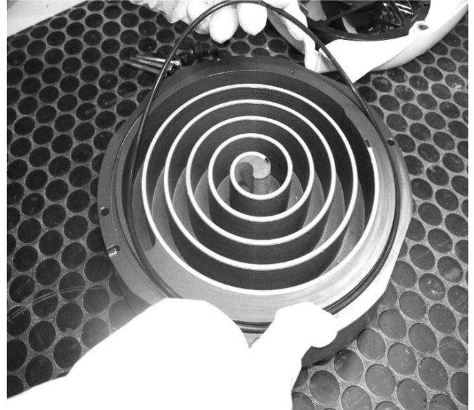
13. Reinstall the outboard housing, making sure the O-ring does not fall out of its groove; secure using the four M4 screws.
